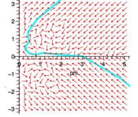
Field plot for the direction of the geometrical tangent to the trajectories, for the values  $\sigma^2=2,\,h=1/8,\,{\rm and}\,\,d=-1.$
