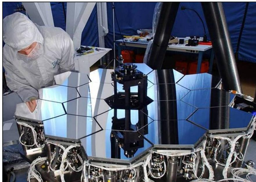
Using a 1/6<sup>th</sup>-scale engineering model to test and validate the algorithms.
