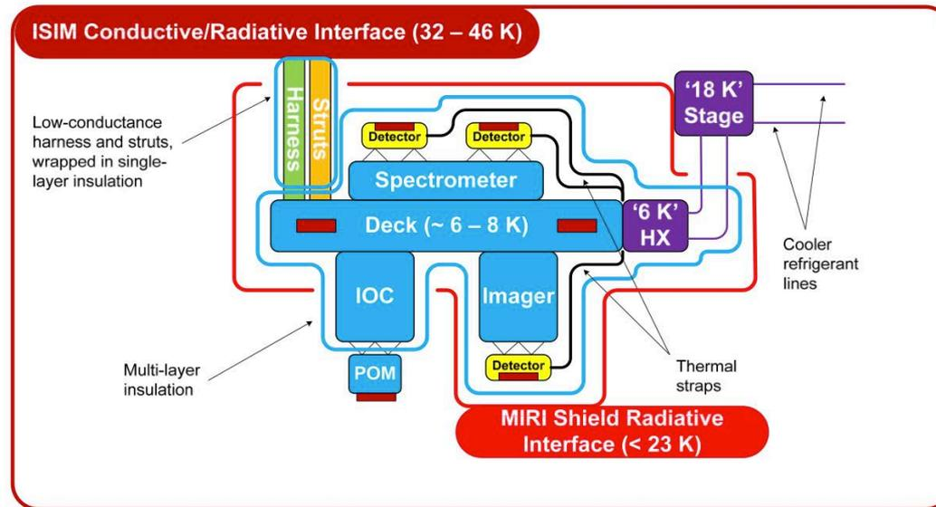
■ = Heaters      △ = Thermally isolating mounts
