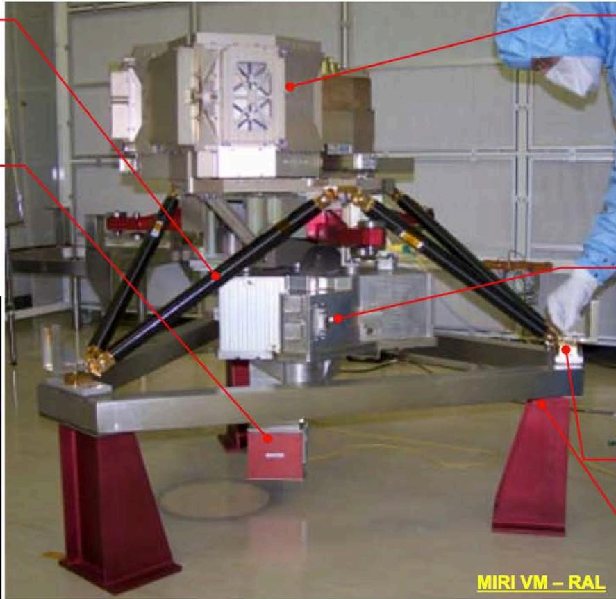
**A 10 x 10 arcsec field passes through the deck into the R ~ 3000, 4 channel integral field spectrometer
