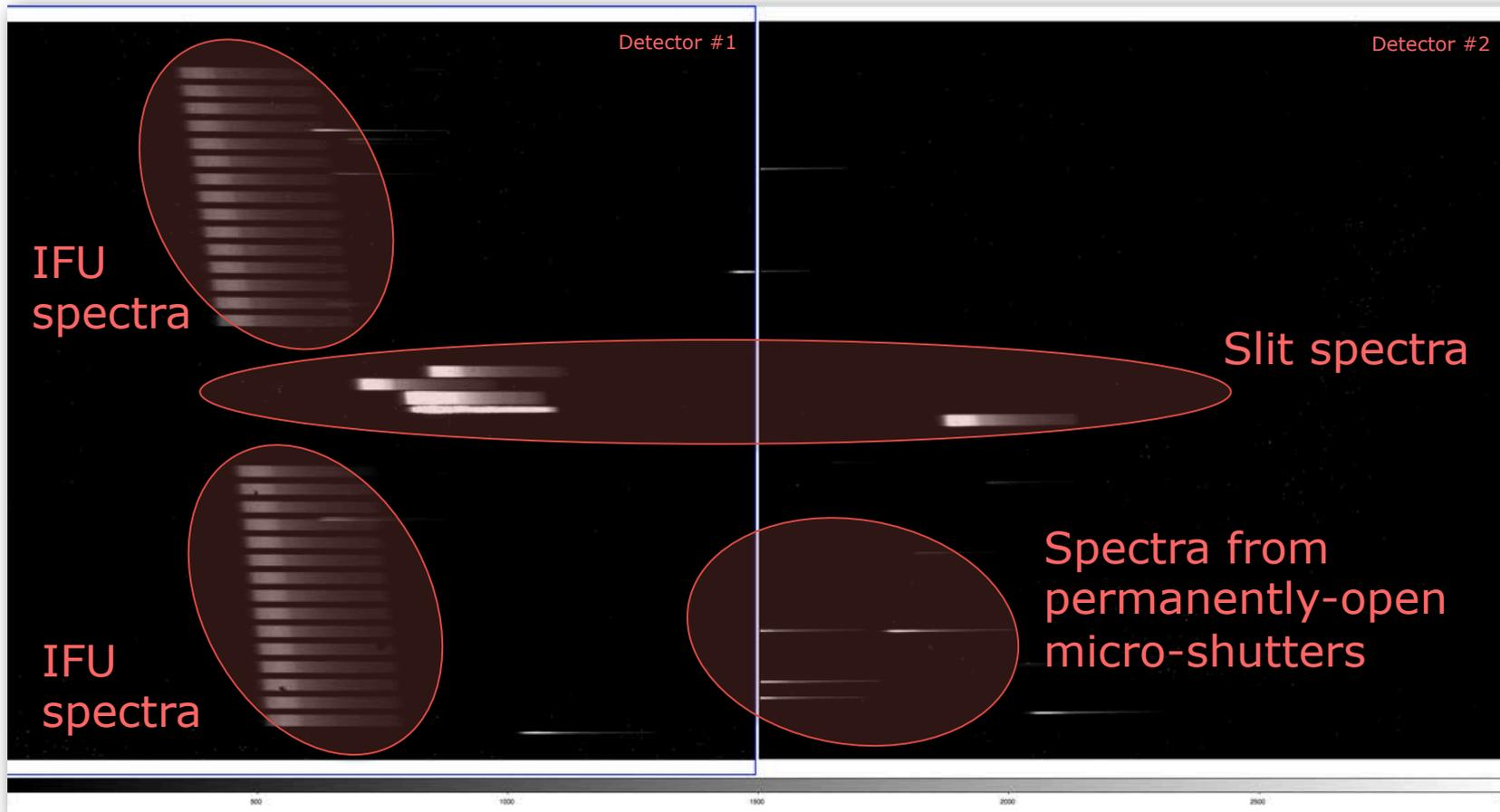
Short continuum spectra obtained with the prism during cryogenic testing in 2011. IFU and SLIT modes.
